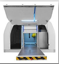
Sliding Load Tray provides additional flexible load capacity, plus additional support for the vehicle operator..
